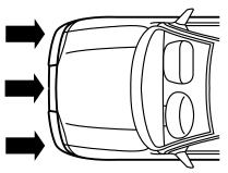
cause activation. Front airbags are designed to activate in frontal and near-frontal collisions, not rollover, side-impact, or rear-impacts unless the collision causes sufficient longitudinal deceleration.
